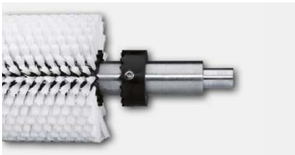
The Multi-Zack segments are positioned and secured on the shaft with the appropriate Multi-Zack adjusting rings. The tothing ensures the drive and the torque transmission.
